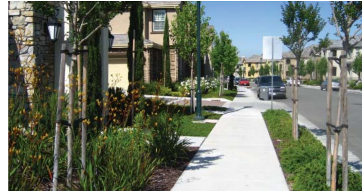
Example of separated sidewalks on a residential street
