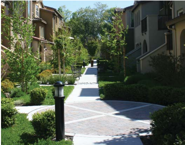
Example of using bollard lighting to highlight pedestrian walkways to individual units
