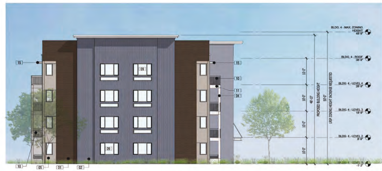
3 BLDG. A - EAST ELEVATION 1/8" = 1'-0" A-02.2
