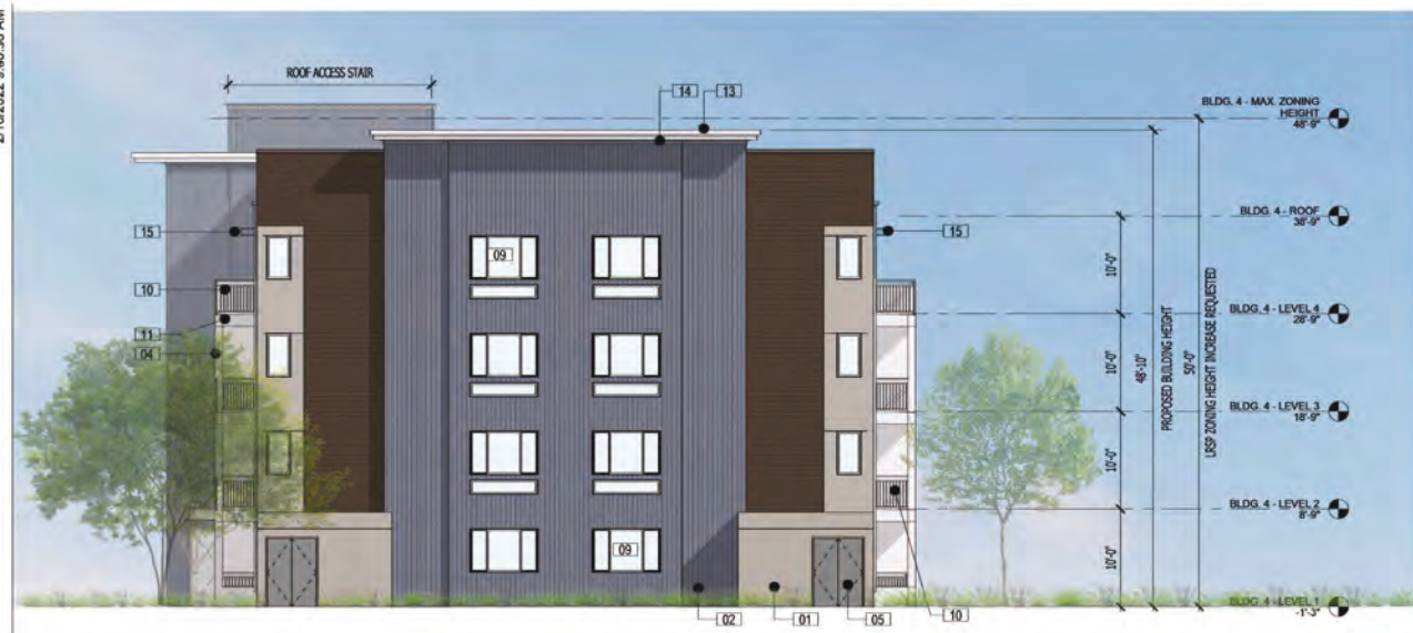
4 BLDG. A - WEST ELEVATION 1/8" = 1'-0" A-02.2
