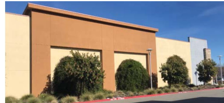
Blank facades should be avoided through change in planes, materials, colors, and landscaping
