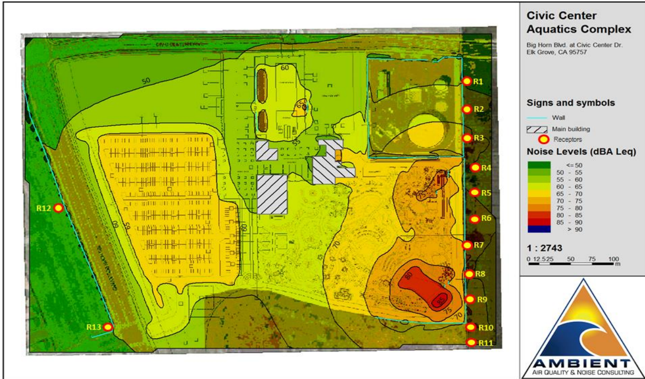
Parking lot noise levels represent Saturday pk-hr conditions. All locations are approximate. Based on site plan dated May 14, 2014.
