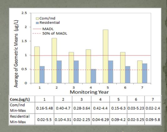
Average geometric mean (min/max) PCP; Sample size = 30
