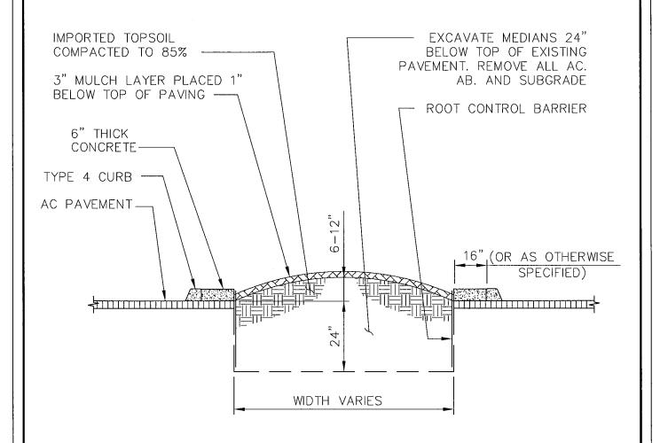
NOTE: CONTOUR OF MEDIAN WILL VARY DEPENDING UPON MEDIAN WIDTH. DO NOT EXCEED BID QUANTITY OF IMPORTED TOPSOIL TO ACHIEVE 12" HEIGHT.
