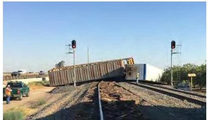
Derailed from railway buckling occurred in Tulare County in 2017
