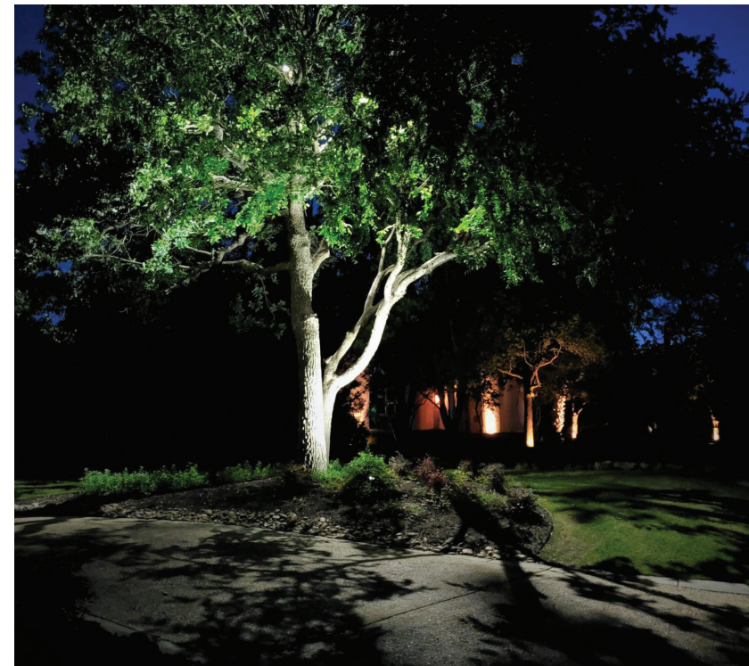
Adjustable luminaires mounted in trees for a downward moonlighting effect at large feature trees along main pathway.
