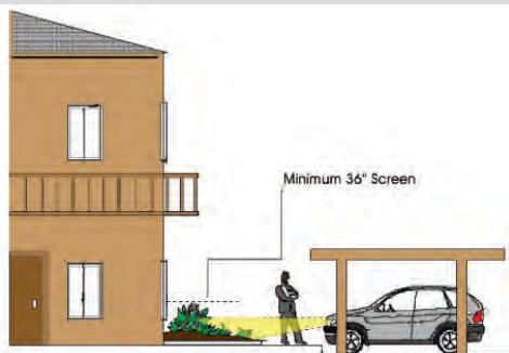
Figure IV-6: An example of landscape with berming used to achieve a minimum 36" screen to shield vehicle headlights from livable portions of the units.
