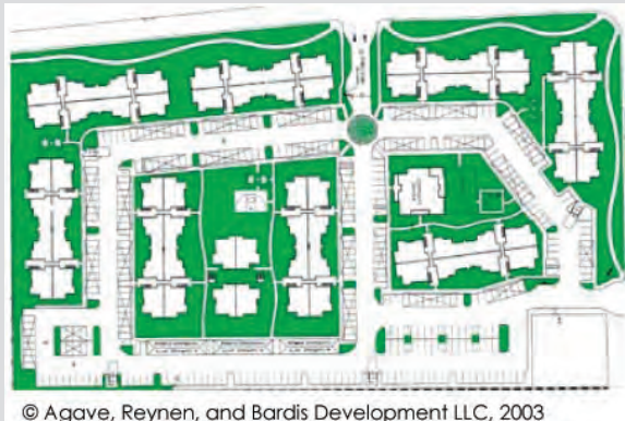
Figure IV-3: Qualifying common space for the purpose of calculating open space is indicated in green.
