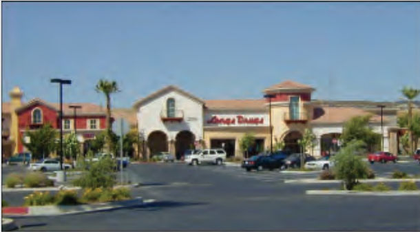
Photo V-46: This development uses articulation , façade , and rooftop variation to achieve a pedestrian scale and reduce the mass of larger tenant spaces.
