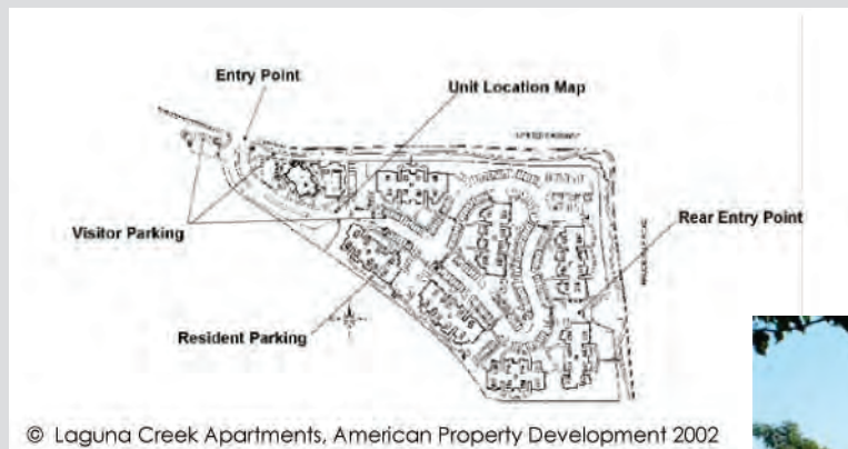
Figure IV-4: Simple internal driveways, unit mapping system and a variety of visitor and resident parking allows for ease of circulation.
