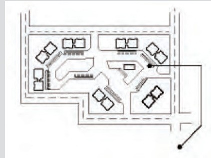
Figure IV-5B: This figure depicts acceptable parking lot design using a series of smaller lots throughout complex.
