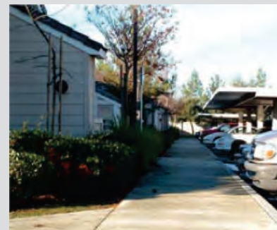
Photo IV-10: This photo shows how landscaping can be used to shield car headlights from shining into living areas of dwelling units.
