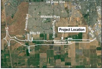
features will include utility relocation, drainage improvements, signalized intersections, and frontage roads. Dependent upon funding, the implementing agency may construct all or part of this Project. Should construction phasing of the Project be necessary, initial construction may consist of a two-lane facility; however, other construction phasing may be considered. The City and Connector JPA are proposing to use funds from FHWA for this local roadway Project.
